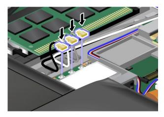
Note: If the new wireless LAN card has two connectors, put the white cable in the cable protection tube.
